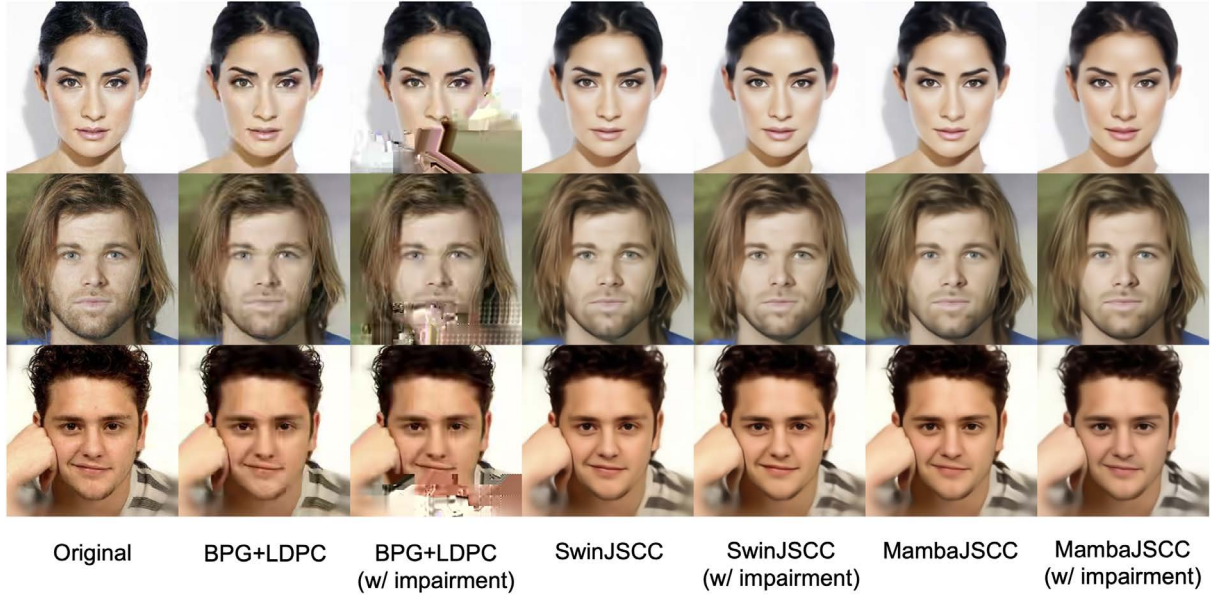
Fig. 6: Visualization of images samples for different schemes transmitted over the AWGN channel (SNR = 10 dB).
