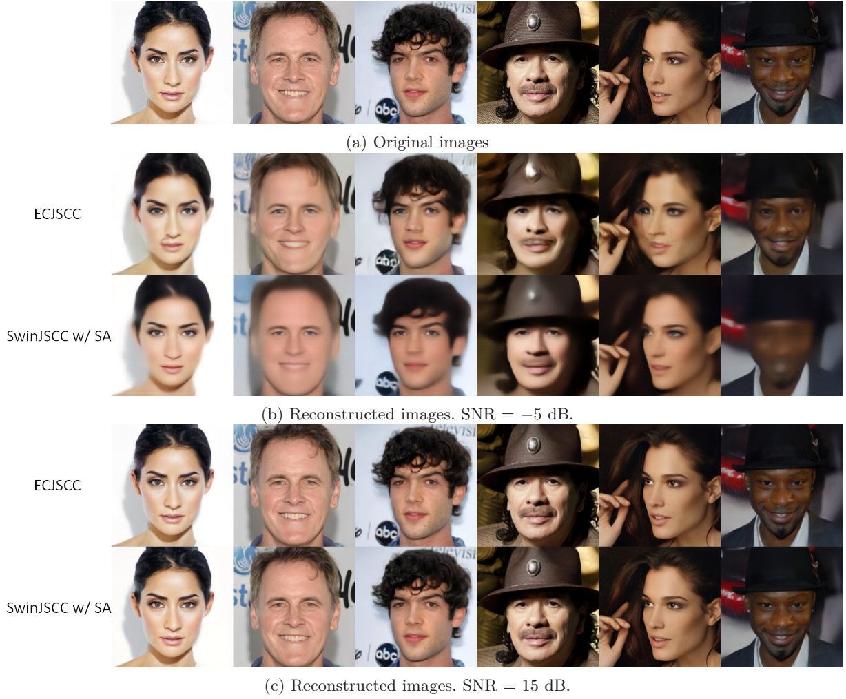
Fig. 5: Comparison of reconstructed images of the proposed ECJSCC with SwinJSCC over the AWGN channel. CelebA-HQ dataset. CBR = 1/32.
